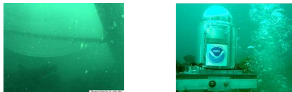
Figure 4. Underwater webcam capable of pan, tilt, zoom and providing streaming video. The camera is located on the Montana shipwreck
