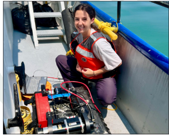
Emma Johnson aboard the R/V Laurentian deploying a radiometer system to measure light in the water column. Photo: Emma Johnson
